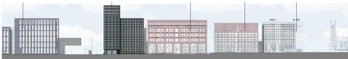
Glenbrook Grey brickwork with curtain wall in fill panels
