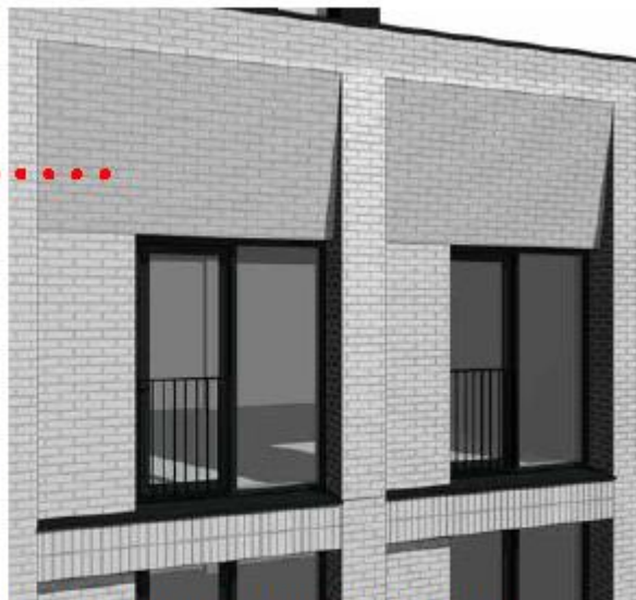
Brick soffit detail to Ellesmere Street Elevation
